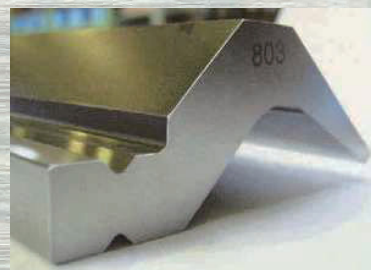
高精度加工が要求されるアイクランプ用金型のベベル溝 Bevel slot of the tool for a I clamp that highly accurate processing is demanded
